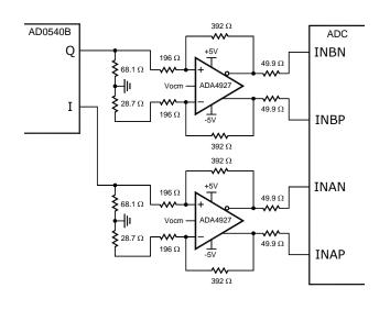
Figure 1. Differential ADC Interface
